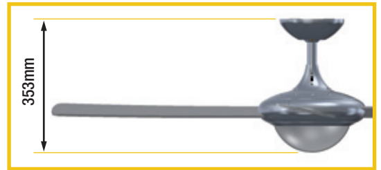
Dimensions of fan with Light Kit
