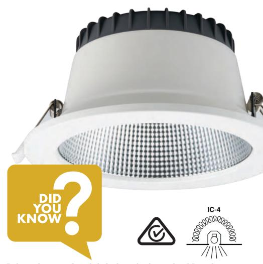
Be fore selecting a downlight look out for the marks of Compliance and Safety. Starting with the RCM mark, this signals that the product has been tested to all relevant Australian Safety standards, to ensure the product delivers its designed safety performance. In addition and when the rmal insulation batts are installed in the ceiling cavity, look out of the IC rating to ensure the product is suitable for such an application.
