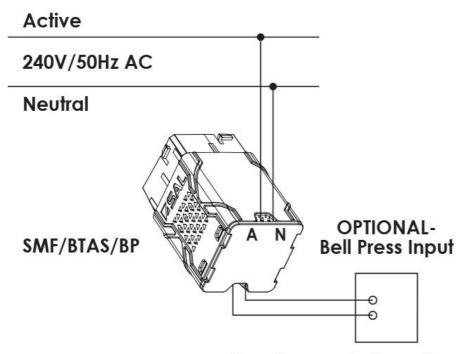
There is no polarity on the bell press conductors.
