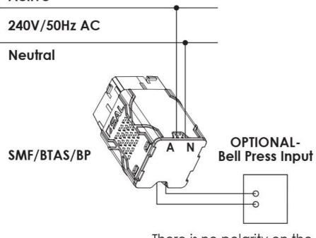
There is no polarity on the bell press conductors.
