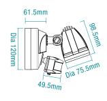
**DOUBLE HEAD** SENSOR AND NO SENSOR
