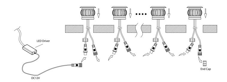
All low voltage products that specify an input of 12v or 24v DC must be used with a suitable LED driver, refer to pages 267 - 274 Lumen output measured at source. All globes supplied with fittings are non dimmable. If you require 240v dimmable globes refer to page 336
