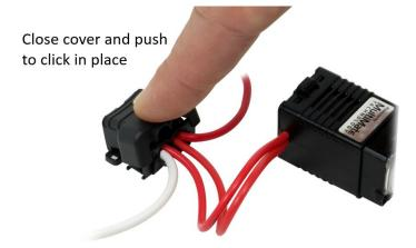
The terminal block can then be cable-tied to the rear of the switch utilising the two loop holes to the housing.
