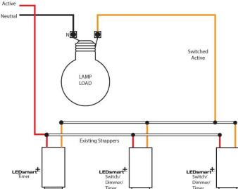
Rocker switches and intermediate switch replaced with LEDsmart<sup>+</sup> devices. The existing strappers are used to connect the devices in parallel. No new wiring is required.
