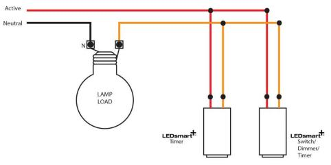
Two-way control using a LEDsmart<sup>+</sup> timer and a dimmer, switch or another timer. Note these two-wire devices are simply connected in parallel.
