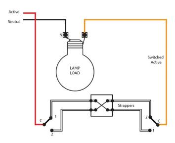
Traditional three-way switching using two rocker switches and one intermediate switch, with strappers between the switches.
