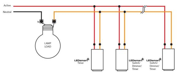
Three-way control using LEDsmart<sup>+</sup> devices. Note that each two-wire LEDsmart<sup>+</sup> device is simply connected in parallel.
