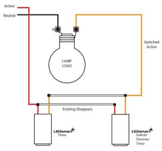
Rocker switches replaced with LEDsmart<sup>+</sup> devices using the existing strapper wires. No new wiring required.
