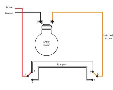
Traditional two-way switching using standard rocker switch mechanisms and strappers between the switches.
