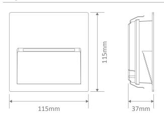
Cutout without recessed box: (L) 100mm x (H) 100mm Cutout with recessed box: (L) 110mm x (H) 110mm
