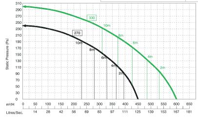
Blizzard has been tested to perform under long ducting, and the resulting chart shows that the airflow (with 10m ducting) still remain reasonably well at around 50% of peak extraction.
