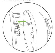
Contacts locate into 3-way terminal block for speedy connection.
