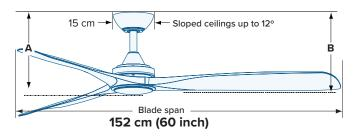
A: 28 cm CEILING TO BOTTOM OF MOTOR LIGHT KIT ADDS 2CM B: 28 cm CEILING TO BOTTOM OF BLADES
