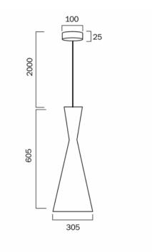
All representations within this document are subject to copyright. ELECTRICAL INSTALLATIONS MUST BE PERFORMED BY A QUALIFIED ELECTRICAL CONTRACTOR AND INSTALLED IN ACCORDANCE WITH AS/NZS 3000. NOTE : All images , descriptions and dimensions are indicative. Please check latest version of item detail on Telbix website prior to ordering or installation.
