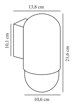
Voltage (V): 220-240 Volt IP degree: IP54 Maximum bulb wattage (W): 60 Class (Class 1, Class 2, Class 3): Class 1 (Earth contact)
