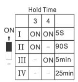
Refers to the time period the lamp remains at 100% illumination after no motion detected.
