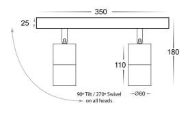
Model NO.: 3A-2142-WH Forging Aluminium Main Material: Finish: **Powder Coated White**
